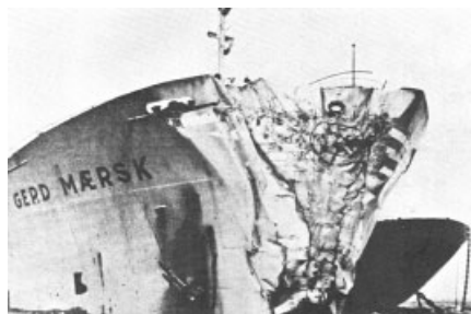
Fig. 2. Newport Bridge, RI, USA, damage to ship
